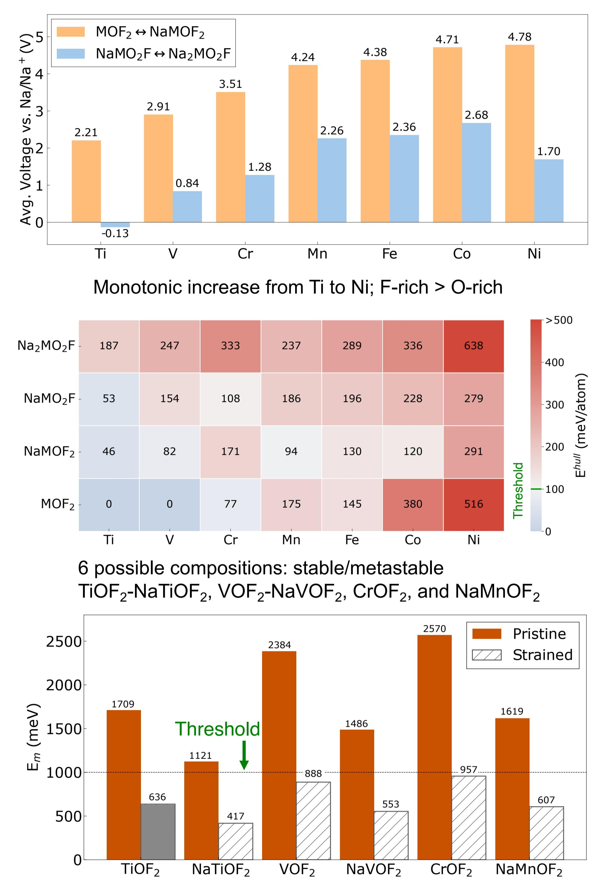
Ti, V, Cr, and Mn oxyfluorides are candidates under strained (thin film) battery geometries
