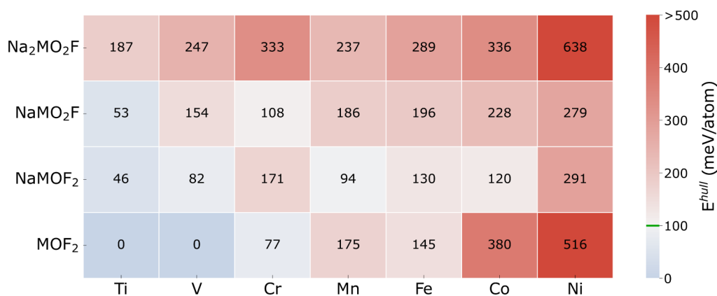
Figure 7. Calculated E^{\text{hull}} for charged and discharged F-rich TMOFs (bottom two rows) and O-rich TMOFs (top two rows). Each column represents a 3d TM, while the E^{\text{hull}} for each compound is indicated by using text annotations within each square. The green line on the legend bar indicates the 100 meV/atom synthesizability threshold considered in this work.
