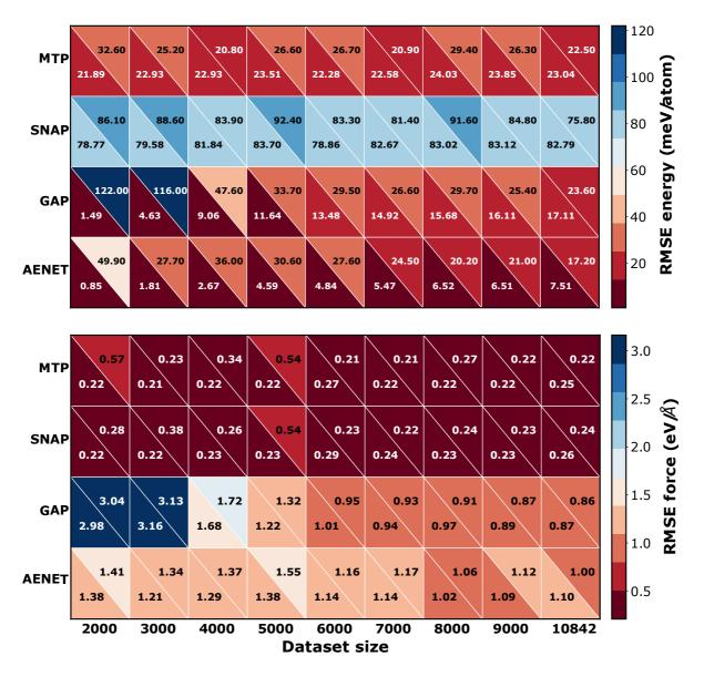
**Figure 3.** RMSE in energies (top panel) and forces (bottom panel) for the MLIPs considered in this work, as a function of increasing total dataset size. Lower left and upper right triangles within each square represent training and test errors, respectively.
