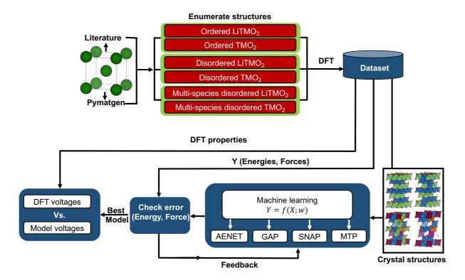
Figure 2. Workflow of structure enumeration, DFT calculations, MLIP training, and voltage predictions employed in this work.
