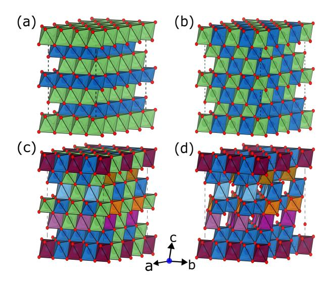
**Figure 1.** Structural schematic of (a) layered LiTMO<sub>2</sub>, (b) disordered, single-TM LiTMO<sub>2</sub>, (c) disordered multi-TM LiTMO<sub>2</sub>, and (d) disordered, delithiated, multi-TM TMO<sub>2</sub>. Green spheres/polyhedra indicate Li, red spheres indicate O, and TMs are indicated by other colors of spheres/polyhedra.
