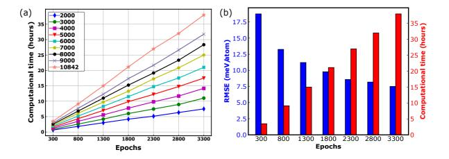
**Figure 5.** (a) Computational training time (in hours) versus number of epochs for different total dataset sizes using AENET. (b) Training energy RMSE (left y-axis and blue bars) using AENET for the total 10842 dataset with increasing number of epochs, with the corresponding computational training time (in hours) also indicated (right y-axis and red bars).
