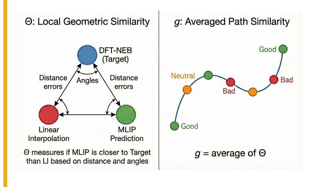
• For a given system containing i intermediate images,  $g = \frac{\Sigma_i \theta}{\Sigma_i i}$
